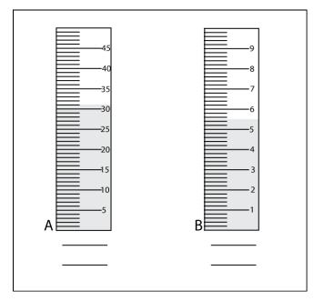
3) Read both of these cylinders. Determine what each line (increment means). These units are milliliters (mL).
